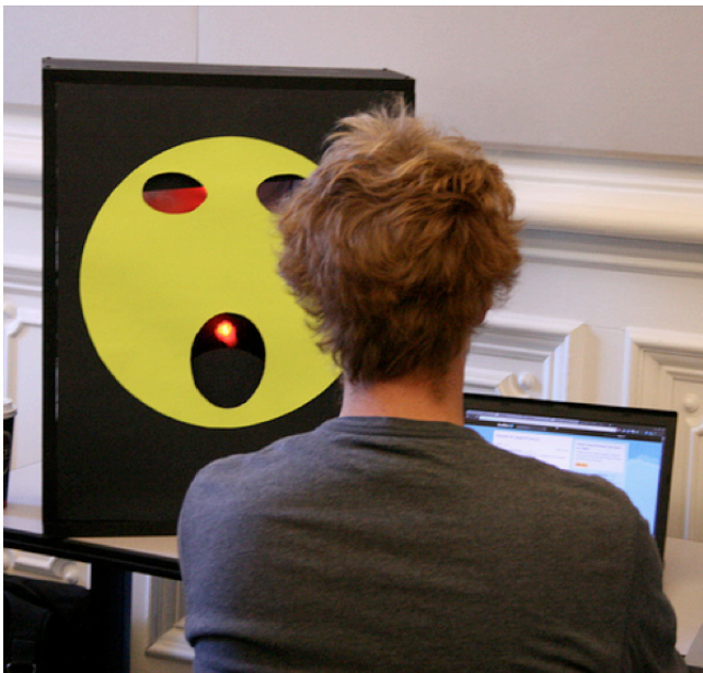
Figure 2. A user interacting with the ambient feedback system that is monitoring the user’s online browsing behavior.
